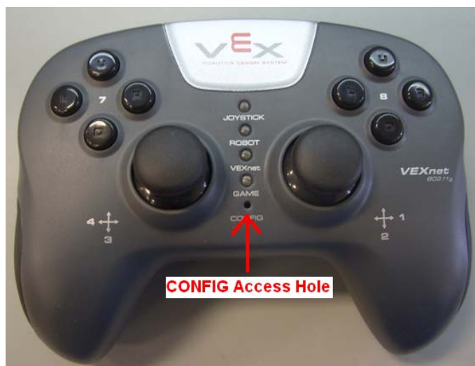
i. VEXnet Joystick CONFIG Switch Access Hole
